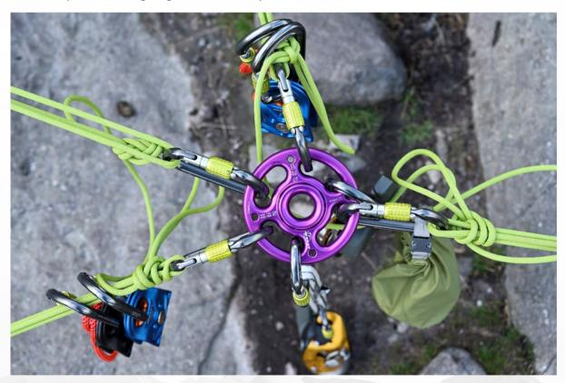
The typical method for building a system utilising these cords involves each anchor leg being built from three strands which form a tensioning system, the tension is taken in equally on all the anchor legs and they are tied off individually.
