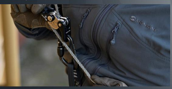
System contains a pre-rigged descent/lowering system. This uses 23m of 5.5mm heat resistant aramid rope with a rigging carabiner, a rope protector and an auto-locking, load limiting rope controller all attached and ready to deploy. Optional extra equipment is available including an ascending system; an ANSI rated rescue hook and aramid sling that increase the options for creating safe anchor points.
