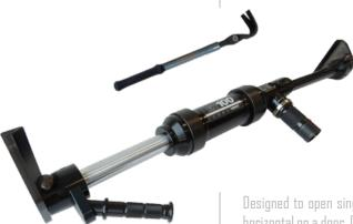
Designed to open single or multi-points anti-panic doors the EXIOO is placed at the horizontal on a door. Once in place, activate the tool with the contactor on the service handle or with a remote control until the jack retracts and squashes the door. The NPB pry bar is used to ease the EXIOO plates positioning.
