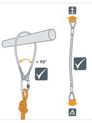
Performance and ultimate strength will be reduced by larks footing / choking around anchor points, storage and ageing due to use, etc. (list not exhaustive).
