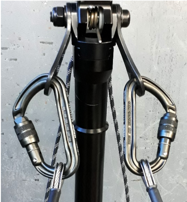
Figure 5: Carabiners connected properly
