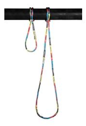
Compact Slings are excellent anchor slings and safety lanyards for rescue and rope access. Strong, durable, and easy to use, they are rated for a four-person load with a 100 kN MBS (end to end configuration). The High Tenacity Polyester (HTP) fiber core makes the Compact Sling highly durable and robust. An elastic polyester sleeve surrounds the internal load bearing elements for added protection, compact sizing, and easy handling.
