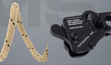
A custom 6.5mm aramid/nylon rope forms the basis of the CTOMS system - the rope was the result of much developement to find the balance of performance, cut resistance and durability with the QA and QD devices. The QA can be used for rope ascension, haul and tension systems, self-belay, rope grabbing and force absorption.
