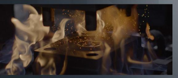
The Ghost carabiner was designed to create a quieter carabiner for covert situations - the Ghost uses a complex hot forged skeleton with an over-molded TPU outer layer. This creates a carabiner with a significantly reduced noise signature.
