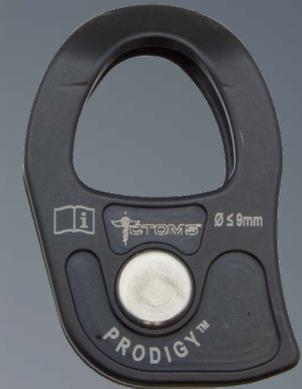
The Prodigy swing cheek micro pulley has a prusik minding edge that allows various MA systems to be created.
