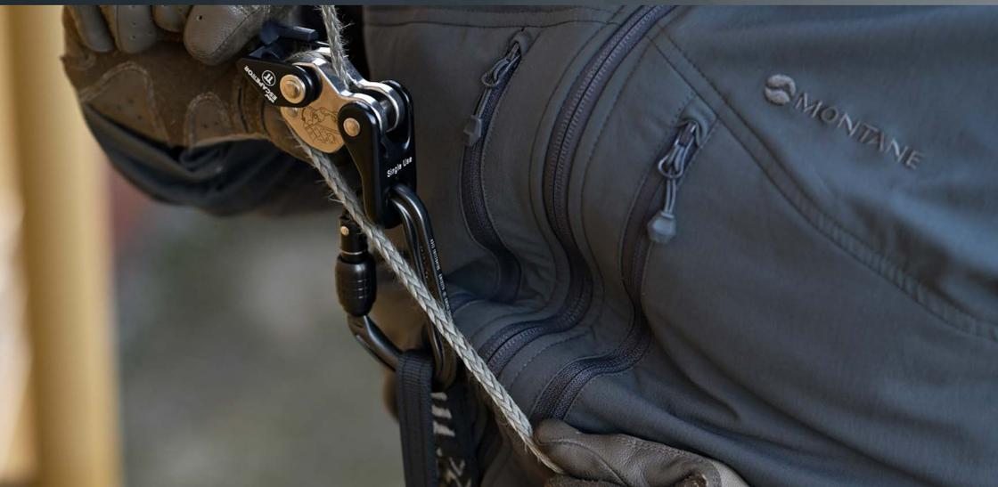
System contains a pre-rigged descent/lowering system. This uses 23m of 5.5mm heat resistant aramid rope with a rigging carabiner, a rope protector and an auto-locking, load limiting rope controller all attached and ready to deploy.
