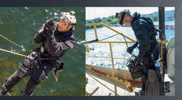
Whether operating at maritime depth, in a desert dust storm,100' AGL in a helicopter, or live bonding transmission lines, the APA-5 is a smaller unit offering a force multiplier that effortlessly reduces time and exposure during vertical operations. Lightweight and powerful, the APA-5 lifts up to 600 lbs directly, handles ropes from 6.5-11mm in diameter, operates at maritime depth, and has a hot-swappable
