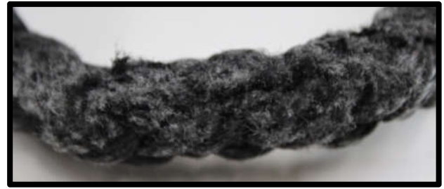
Picture 12: Severe wear of extraction loop.
