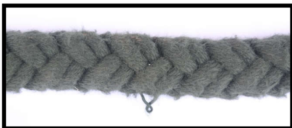
Picture 2: Hooked Yarn under 25mm
