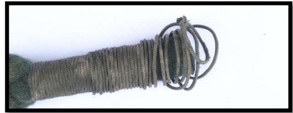
Picture 3: End whipping damaged and must be replaced.
