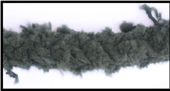
Picture 5: Excessive wear on the rope and should be withdrawn from service.
