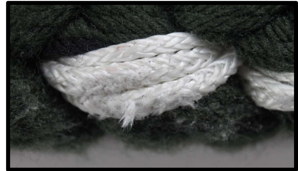
Picture 7: Surface abrasion of DLT termination.
