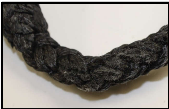
Picture 11: Normal surface abrasion on extraction loop.
