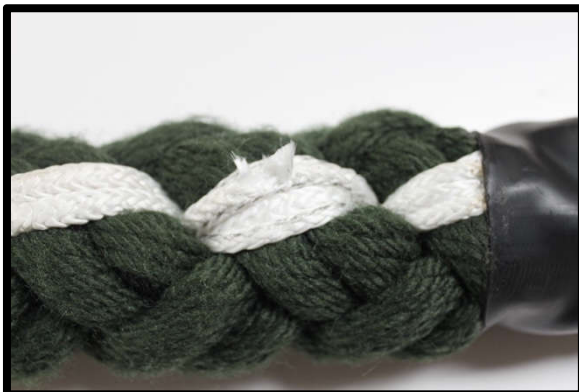
Picture 6: Cut strand on DLT termination.
