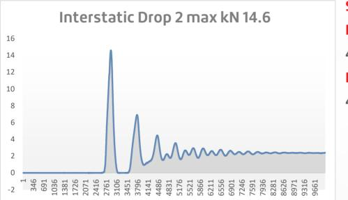
Slip Distance: Rope 1: 45mm Rope 2: 40mm
