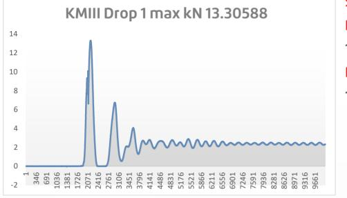
Slip Distance: Rope 1: 165mm Rope 2: 140mm
