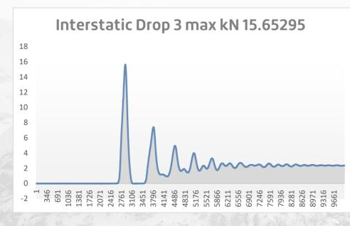
Slip Distance: Rope 1: 35mm Rope 2: 40mm
