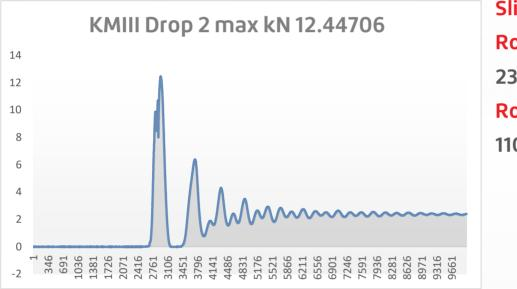
Slip Distance: Rope 1: 230mm Rope 2: 110mm
