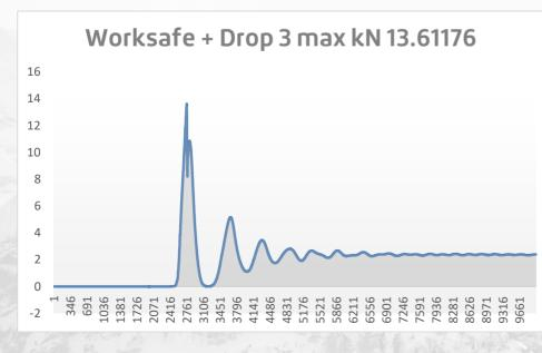
Slip Distance: Rope 1: 60mm Rope 2: 200mm
